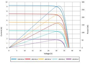
Excellent performance under weak light conditions: at an irradiation intensity of 200 W/m<sup>2</sup> (AM 1.5, 25 °C), **96.5%** or higher of the STC efficiency
